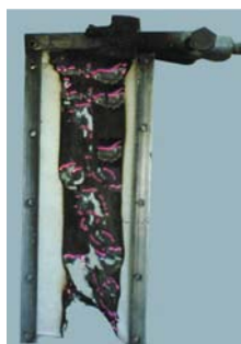
Fig. 2 Mostashari’s Flammability Tester with a low addition of magnesium bromide hexahydrate applied onto a cotton fabric at the end of the experiment
