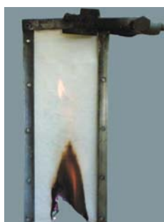
Fig. 1 Mostashari’s Flammability Tester with a low addition of magnesium bromide hexahydrate applied onto a cotton fabric during the test
